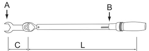
A number of variables including the length of the adapter or extension, length of the wrench and variations in hand position on the wrench will affect the accuracy of the above calculation.
