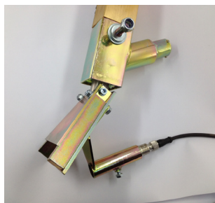
Bead alarm mounted on bead gun
