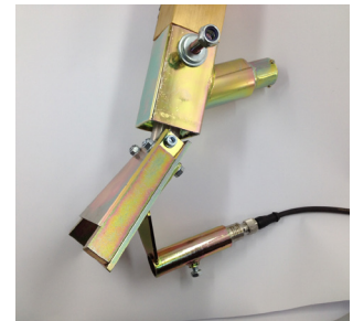
Bead alarm mounted on bead gun
