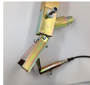
Bead alarm mounted on bead gun
