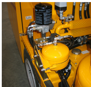
Air drier for bead tank
