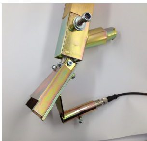
Bead alarm mounted on bead gun
