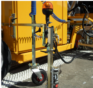
Pre-marking system with paint can
