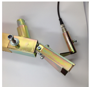
Bead alarm mounted on bead gun
