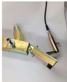
Bead alarm mounted on bead gun
