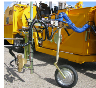
Pre-marking system with paint gun
