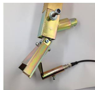
Bead alarm mounted on bead gun
