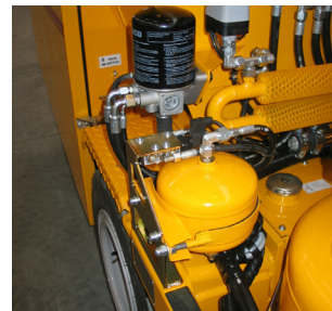
Air drier for bead tank
