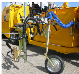
Pre-marking system with paint gun
