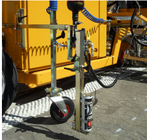
Pre-marking system with paint can
