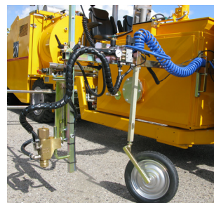
Pre-marking system with paint gun
