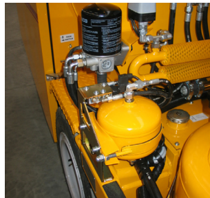
Air drier for bead tank
