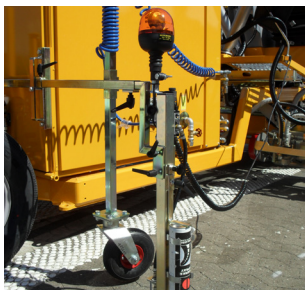
Pre-marking system with paint can
