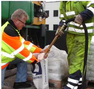
Ejector filling of bead tank
