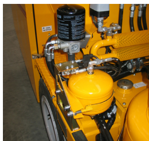
Air drier for bead tank
