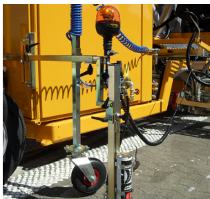
Pre-marking system with paint can
