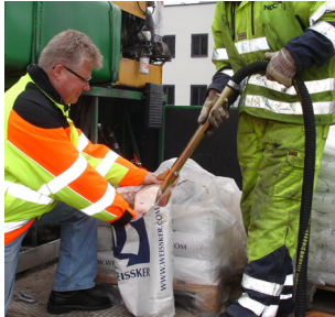
Ejector filling of bead tank
