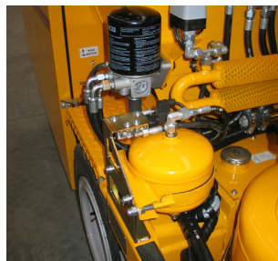
Air drier for bead tank
