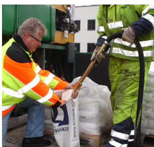
Ejector filling of bead tank
