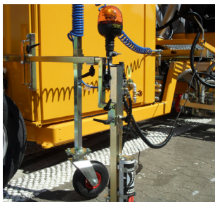
Pre-marking system with paint can
