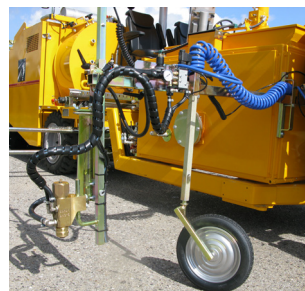
Pre-marking system with paint gun
