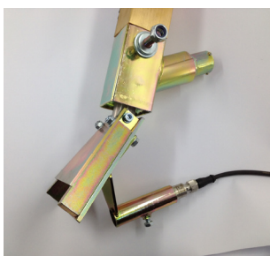
Bead alarm mounted on bead gun
