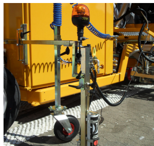
Pre-marking system with paint can
