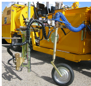
Pre-marking system with paint gun
