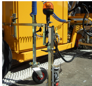
Pre-marking system with paint can
