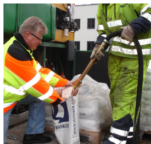
Ejector filling of bead tank
