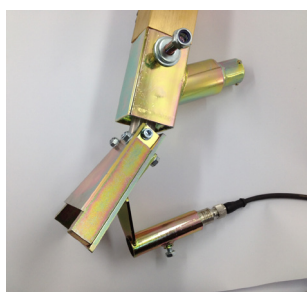
Bead alarm mounted on bead gun
