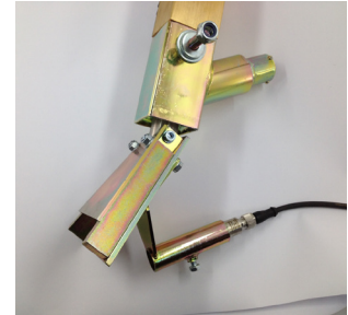
Bead alarm mounted on bead gun
