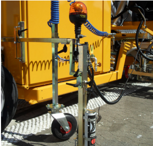
Pre-marking system with paint can
