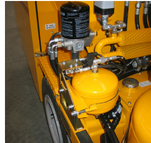
Air drier for bead tank
