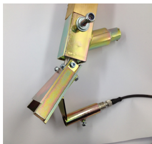
Bead alarm mounted on bead gun
