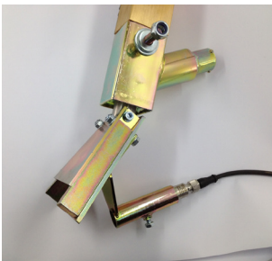
Bead alarm mounted on bead gun
