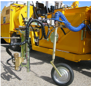
Pre-marking system with paint gun
