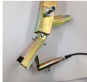
Bead alarm mounted on bead gun
