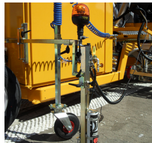
Pre-marking system with paint can
