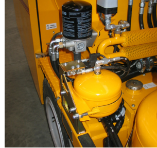
Air drier for bead tank
