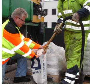
Ejector filling of bead tank
