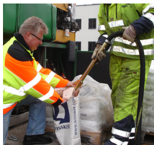
Ejector filling of bead tank
