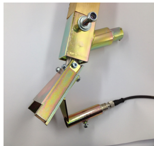
Bead alarm mounted on bead gun
