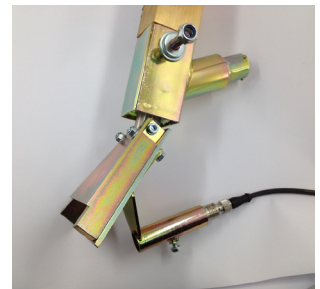
Bead alarm mounted on bead gun
