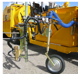
Pre-marking system with paint gun
