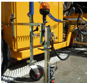
Pre-marking system with paint can
