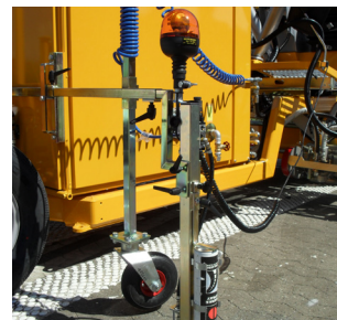
Pre-marking system with paint can
