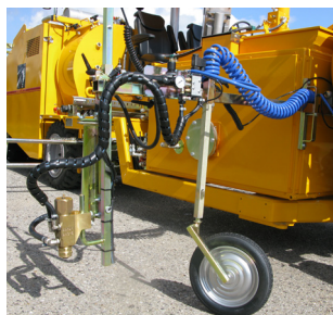
Pre-marking system with paint gun
