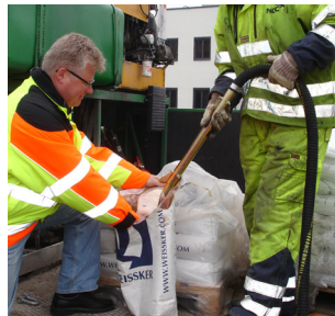
Ejector filling of bead tank
