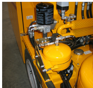
Air drier for bead tank
