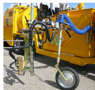
Pre-marking system with paint gun
