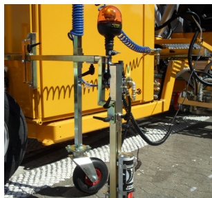
Pre-marking system with paint can
