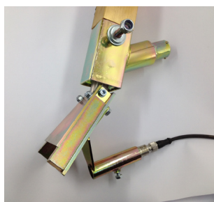
Bead alarm mounted on bead gun
