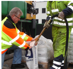
Ejector filling of bead tank
