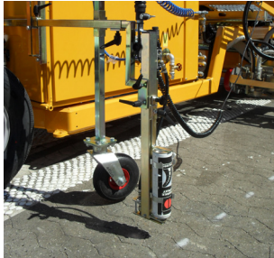
Pre-marking system with paint can
