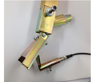
Bead alarm mounted on bead gun
