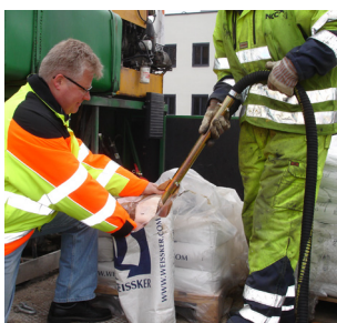
Ejector filling of bead tank
