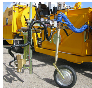
Pre-marking system with paint gun
