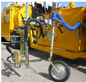
Pre-marking system with paint gun
