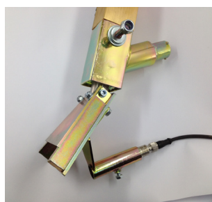
Bead alarm mounted on bead gun
