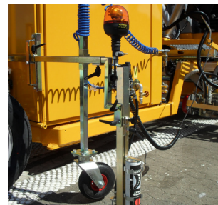
Pre-marking system with paint can
