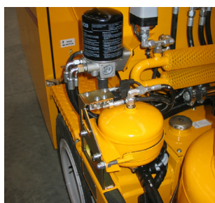
Air drier for bead tank
