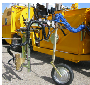
Pre-marking system with paint gun
