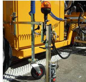
Pre-marking system with paint can
