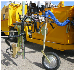
Pre-marking system with paint gun
