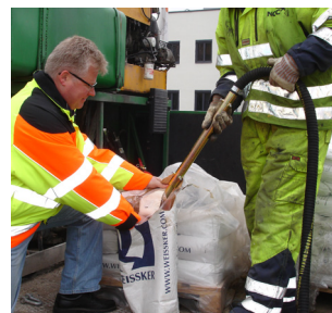
Ejector filling of bead tank
