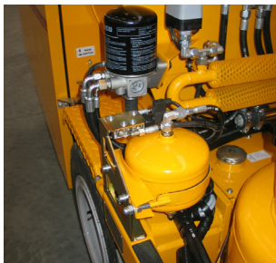
Air drier for bead tank
