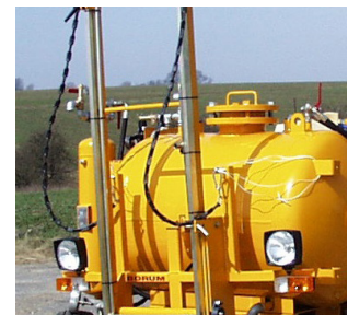
Fixed pointer With hydraulic lifting system
