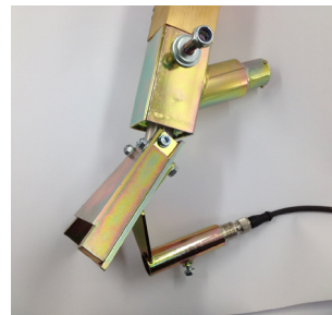
Bead alarm mounted on bead gun
