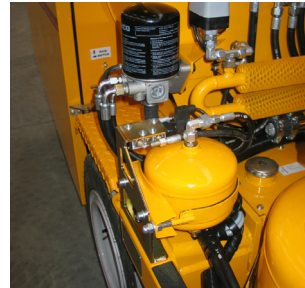
Air drier for bead tank
