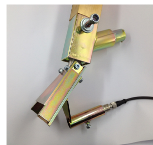
Bead alarm mounted on bead gun
