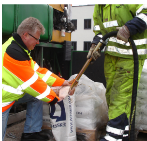
Ejector filling of bead tank
