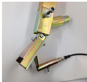
Bead alarm mounted on bead gun
