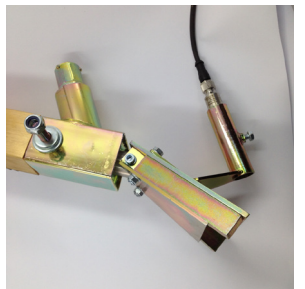
Bead alarm mounted on bead gun
