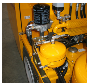
Air drier for bead tank
