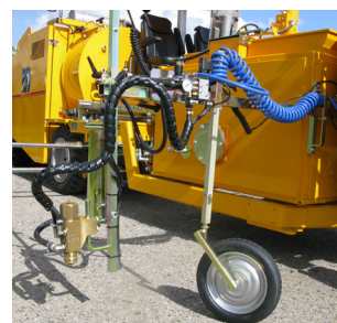
Pre-marking system with paint gun
