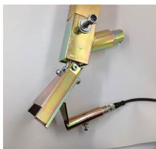
Bead alarm mounted on bead gun
