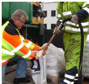
Ejector filling of bead tank
