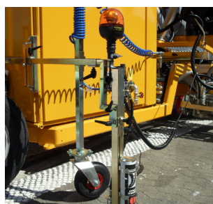
Pre-marking system with paint can
