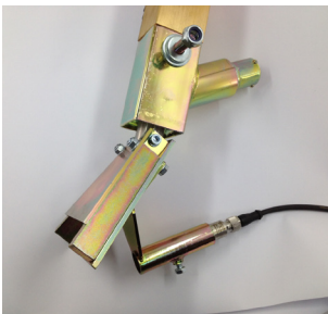
Bead alarm mounted on bead gun
