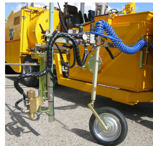
Pre-marking system with paint gun
