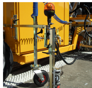
Pre-marking system with paint can
