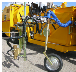
Pre-marking system with paint gun
