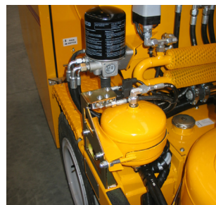
Air drier for bead tank
