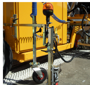
Pre-marking system with paint can
