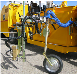
Pre-marking system with paint gun
