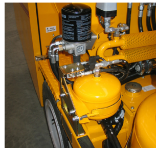
Air drier for bead tank
