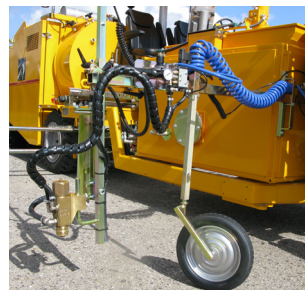
Pre-marking system with paint gun
