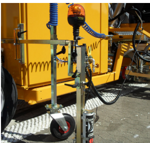
Pre-marking system with paint can
