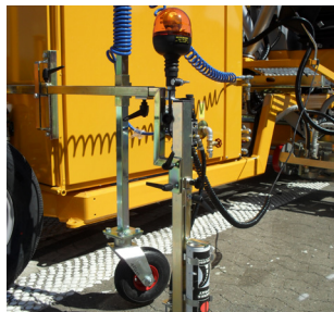
Pre-marking system with paint can
