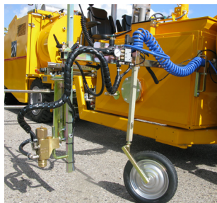
Pre-marking system with paint gun
