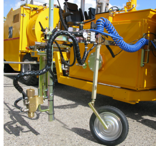
Pre-marking system with paint gun
