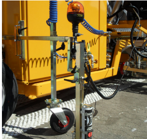
Pre-marking system with paint can
