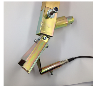
Bead alarm mounted on bead gun
