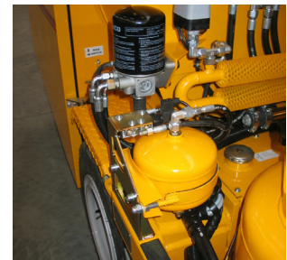
Air drier for bead tank
