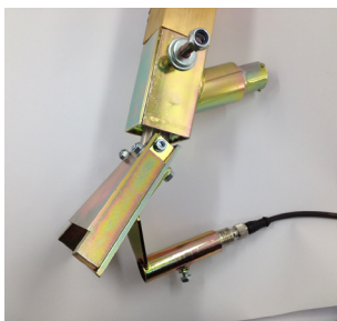
Bead alarm mounted on bead gun
