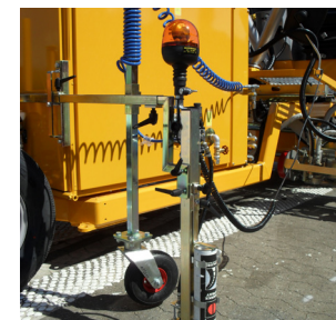
Pre-marking system with paint can
