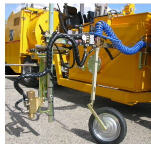
Pre-marking system with paint gun
