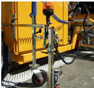
Pre-marking system with paint can
