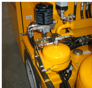
Air drier for bead tank
