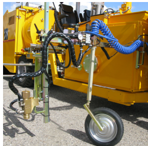
Pre-marking system with paint gun
