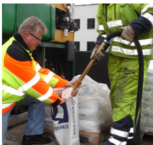
Ejector filling of bead tank
