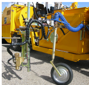
Pre-marking system with paint gun
