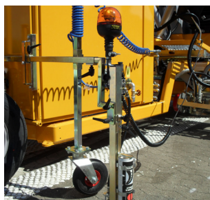
Pre-marking system with paint can
