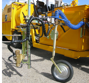
Pre-marking system with paint gun
